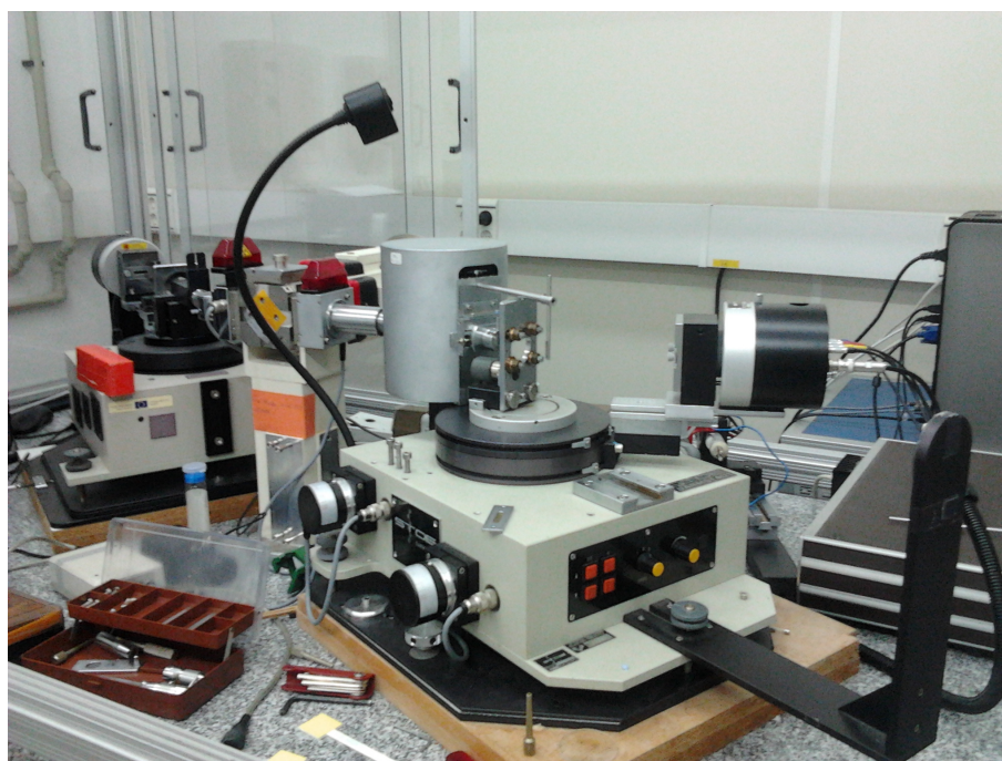
Figure B.4: Stoe STADI-P laboratory X-ray powder diffractometer.
