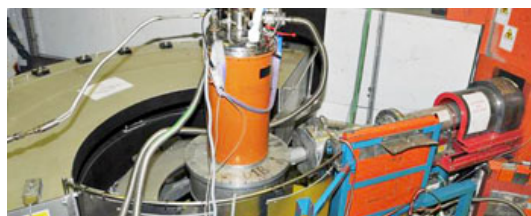
Figure B.13: D1B neutron powder diffractometer.
