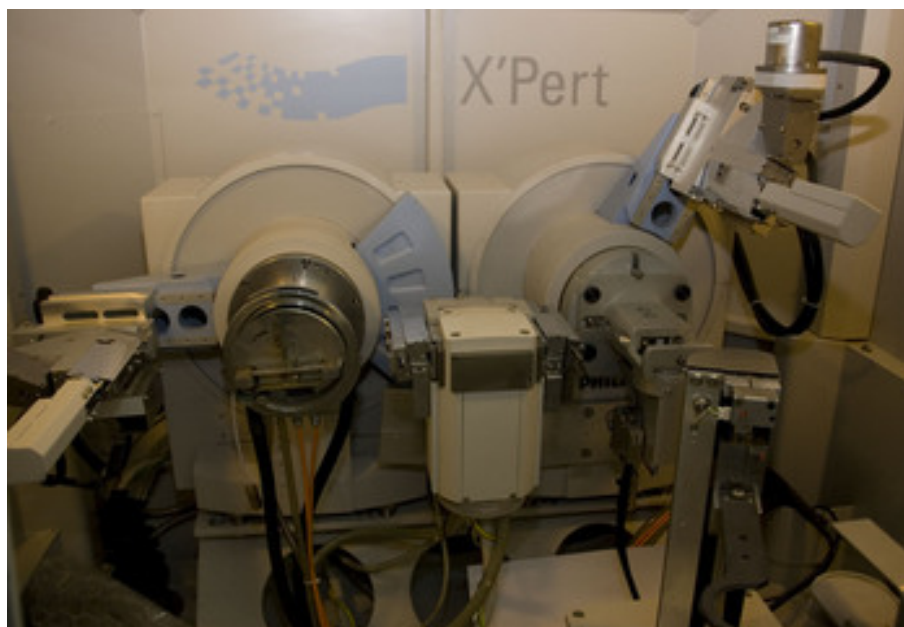
Figure B.5: Philips X'Pert MPD laboratory X-ray powder diffractometer.
