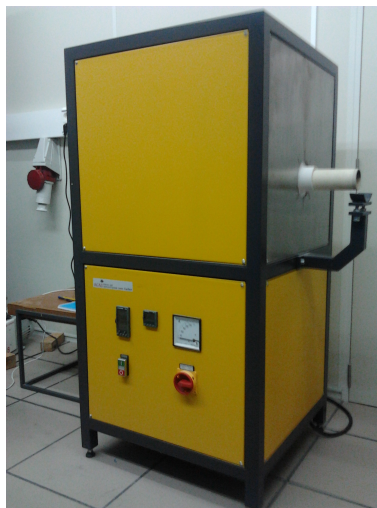
Figure B.3: AGNI Ceram-Aix RHT 175-50-300-1H furnace.
