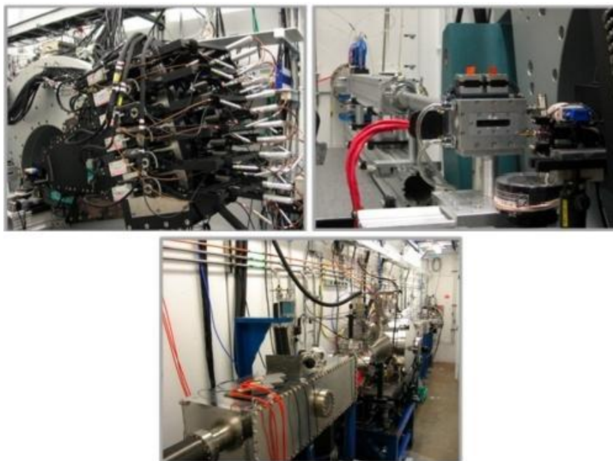
Figure B.8: Powder diffractometer from 11-BM-B line in Argonne National Laboratory Synchrotron.
