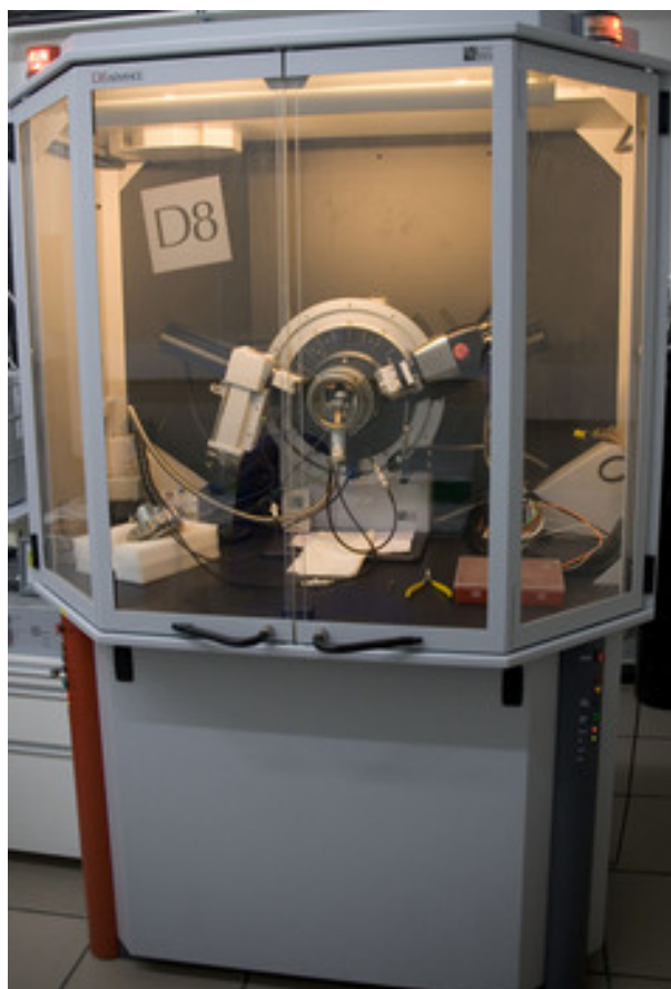
Figure B.7: Bruker Advance D8 Vantec laboratory X-ray powder diffractometer.
