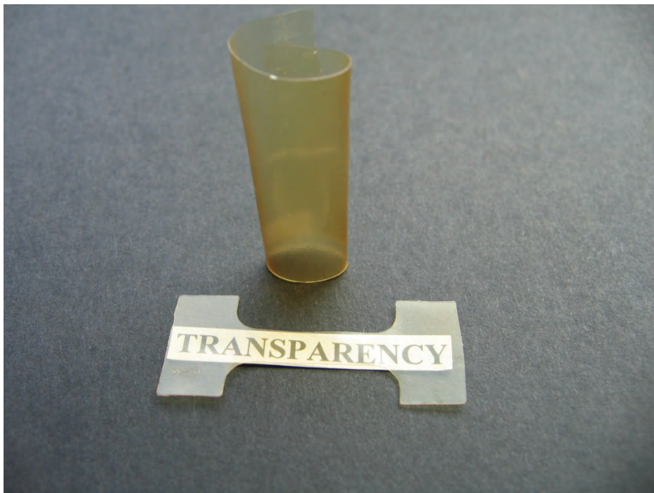
Figure 5.1. Visual aspect of SPI-based films modified with 15% bovine gelatin and processed by compression moulding technique.
