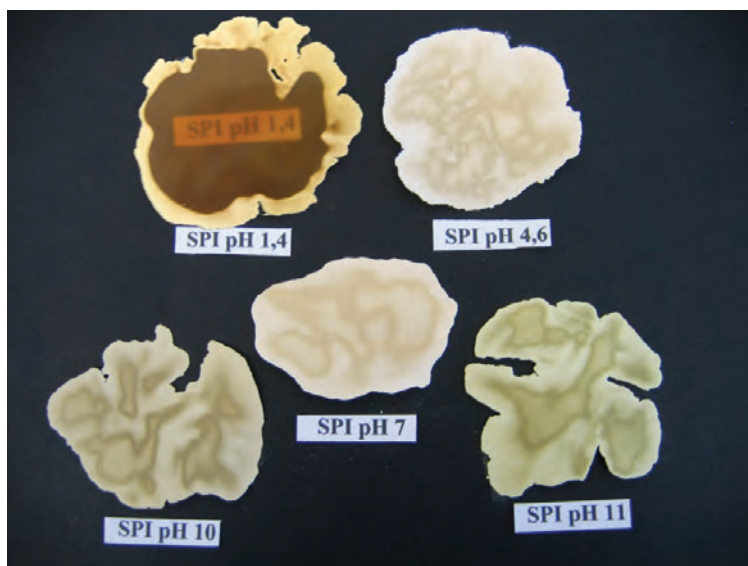
Figure 4.1. SPI films prepared at different pHs, freeze-dried and hot-pressed.
