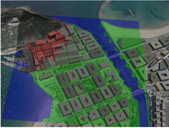
Figure 17: Simulation of a theoretical mixed fire in San Sebastian (Spain). The terrain, the land use and the building information have been constructed from open data sources.
