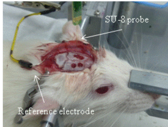
Figure 5.4 In vivo testing using SU-8 microprobes
