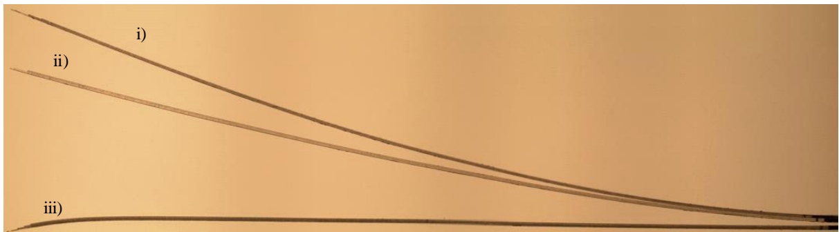
Figure 5.13 The curvature of: i) Four 20 \mu\text{m} thick SU-8 layers processed using the masks based on the first design, ii) two 20 \mu\text{m} thick SU-8 layers and a layer of 40 \mu\text{m} processed using the masks based on the first design, and iii) four 20 \mu\text{m} thick SU-8 layers patterned using the masks with the novel design.
