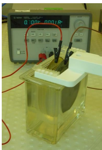
Figure 5.16 A picture of the electrochemical etching set up used for the release of the SU-8 probes
