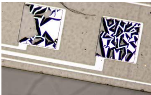
Figure 3.16. Broken electrodes after the activation process
