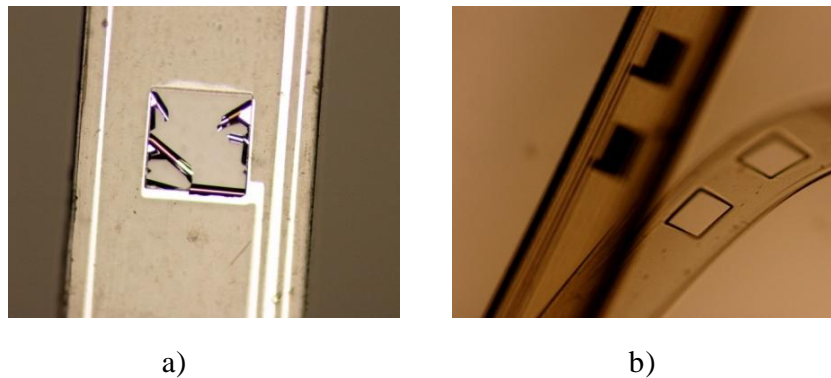
Figure 3.6 a) Broken electrodes after a platinization procedure and b) the passivation SU-8 layer is removed from the bottom SU-8 layer.
