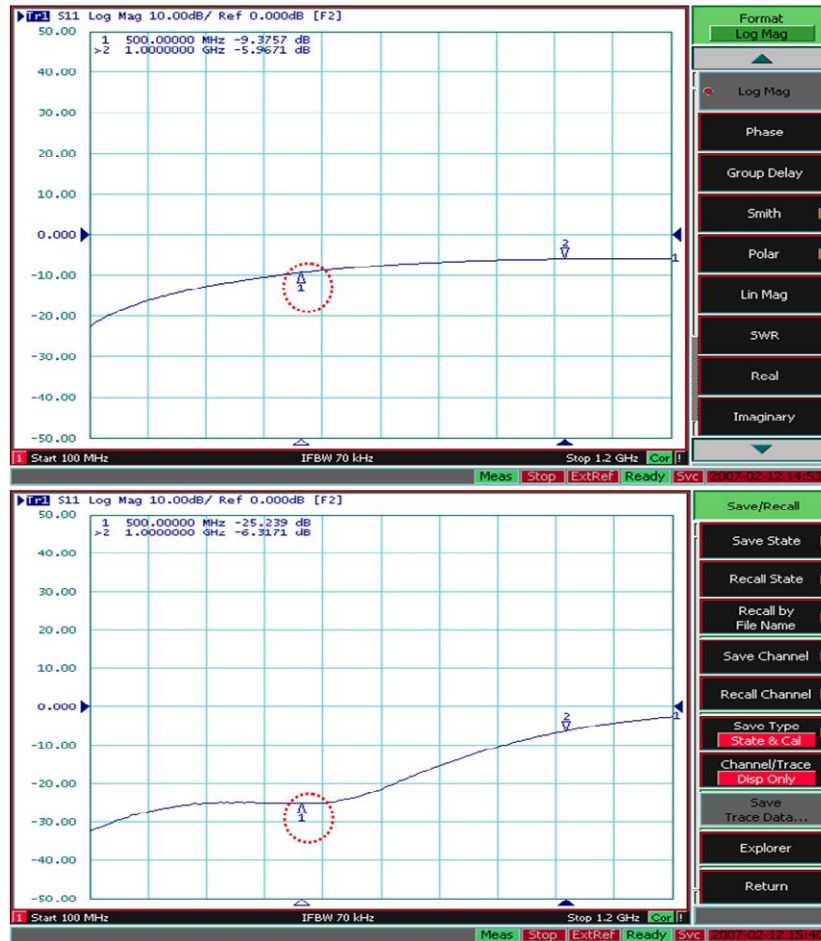
Figure 3.24: Measured S_{11} of the RF_{in} port (500 MHz); Top: before impedance matching; Bottom: 15 dB of S_{11} improvement after impedance matching
