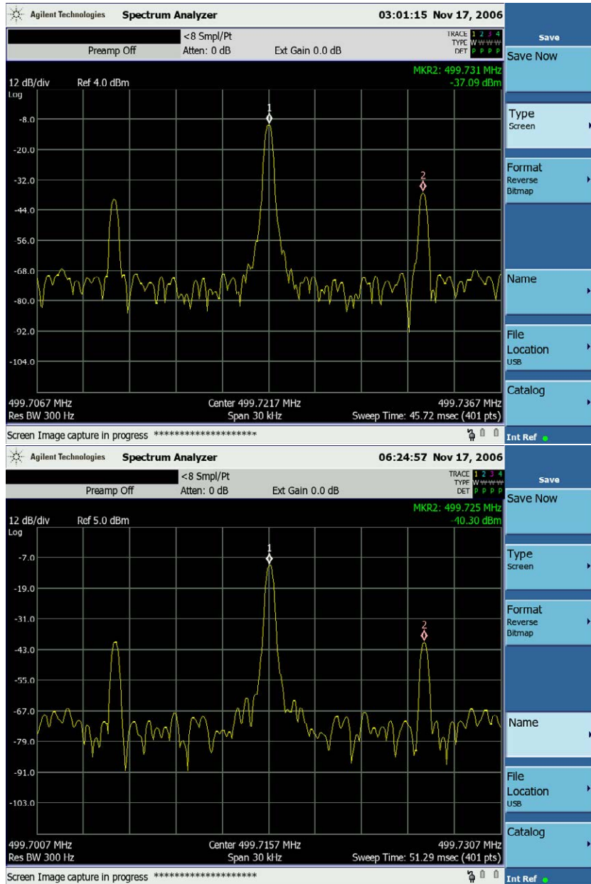
Figure 3.40: Comparison between the PI and PID responses at f_{ripple} = 10 \text{ kHz} ; the ripple amplitude is 3 dB lower with PID (bottom) compared to PI (top).
