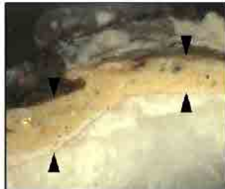
Cross-section from a juxtaposed applied brocade of the triptych of La Asunción-Coronación de la Virgen. The lower (white colour) and the upper (earth colour) layers of the imprimatura are indicated between pairs of arrows. Image width: 425 \mu m.
