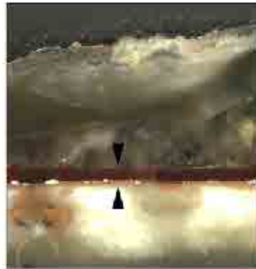
Cross-section from an isolated applied brocade of the triptych of La Asunción-Coronación de la Virgen. The bole (lower layer), the silver leaf (middle layer) and the organic red (upper layer) of the imprimatura are indicated between pair of arrows. Image width: 420 \mu m.
