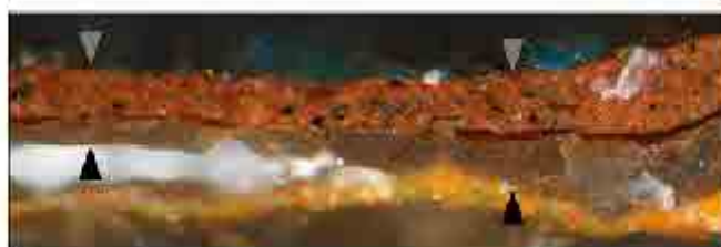
Cross-section of the triptych of San Antón showing (from bottom to top) the tin leaf, the oil layer, the paint layer with multiple inclusions, the oil layer and the gold leaf (the last two layers are not visible because of their extreme thinness). These layers are indicated between pairs of arrows. Image width: 150 \mu m.
