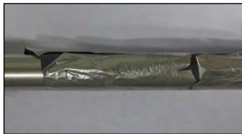
Figure 6.16. M6 membrane peeling off detected at 3600 h.
