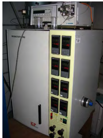
Figure 3.1. Diagram and image of the bench-scale pilot plant PP for catalysts activity tests.
