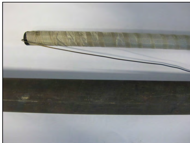
Figure 6.7. Hard chrome plated tube and the “stainless steel membrane” covered with a high temperature tape after performing CPO.
