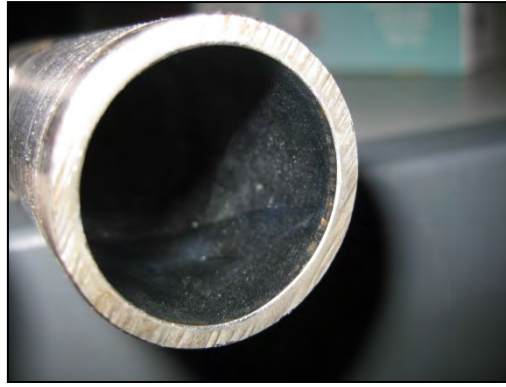
Figure 6.5. Membrane module with the hard chrome plating inside.
