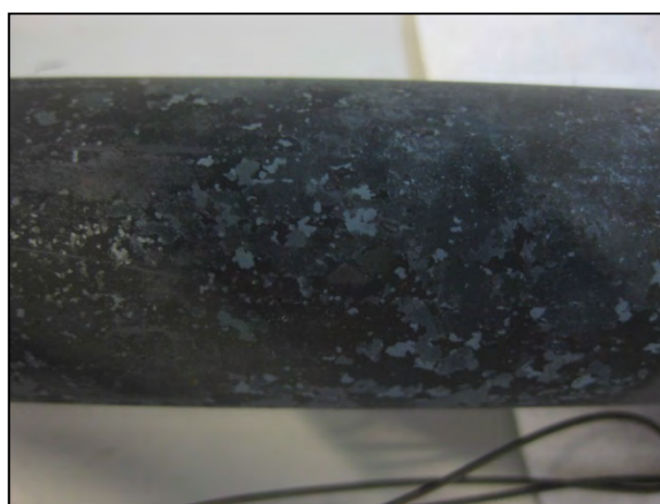
Figure 6.4. The steel tube of the membrane module after tests at 1073 K.
