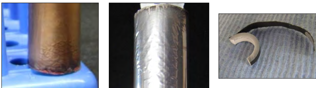
Figure 5.9. Delamination problems could be visually predicted in the membranes before and after Cu plating.
