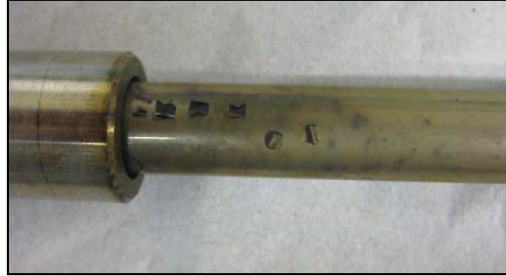
Figure 6.20. Picture of the detached metal layer in the close cap area of the used M7 membrane.
