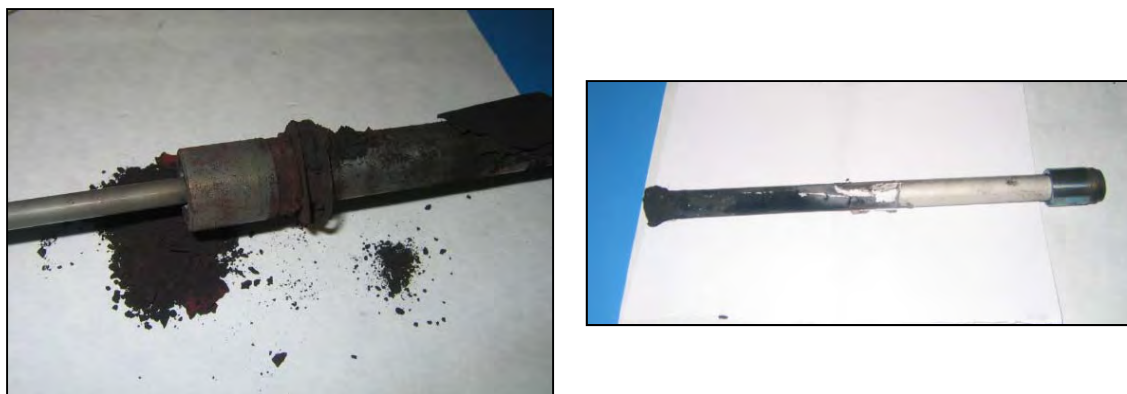
Figure 6.2. Coke formation in the membrane module during the initial tests with complex mixtures.
