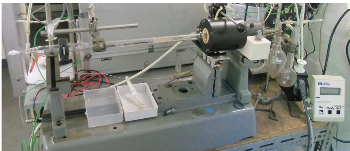
Figure 3.9. Photograph of the fast pyrolysis minireactor
