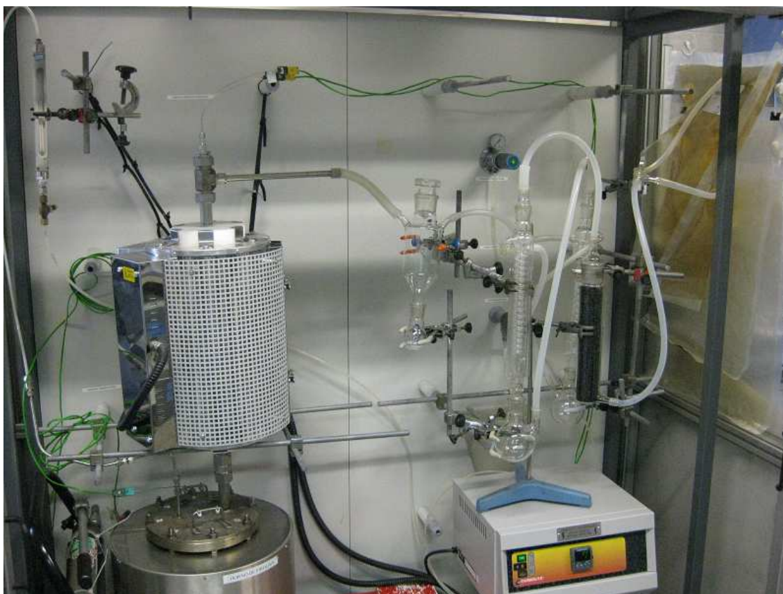
Figure 3.7. Photograph of the slow pyrolysis plant
