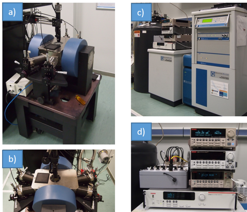
Figure 3.15: Equipment for the electrical characterization. a) and b) Lakeshore Probe Station, side and top view respectively. c) Physical Properties Measurement System (PPMS) from Quantum Design Inc. . d) Example of Keithley moduli for sourcing and/or measuring electrical currents and voltages.
