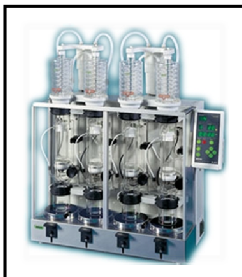
Figure 3.3. Extraction system B-811 (BÜCHI).
