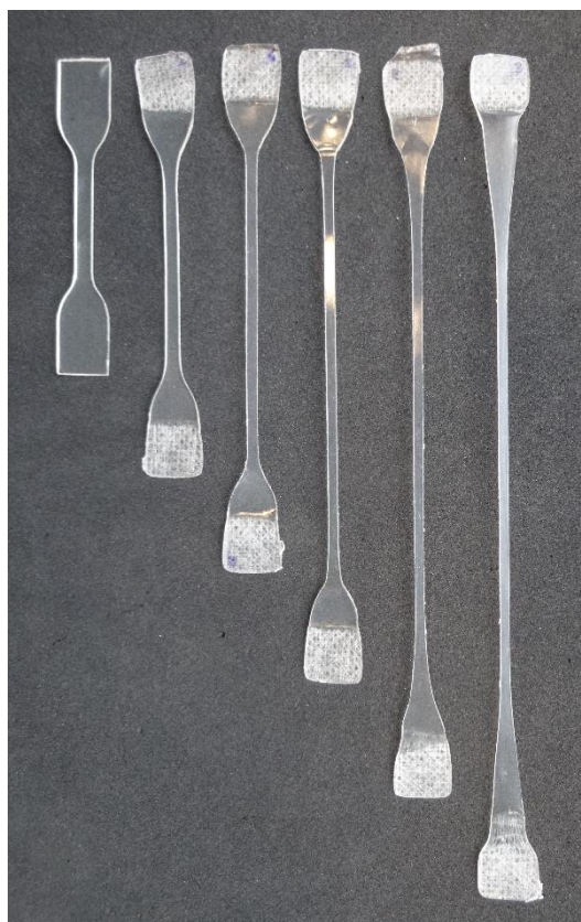
Figure 3.5.- Photographs of unstretched and relaxed samples showing uniform elongation.
