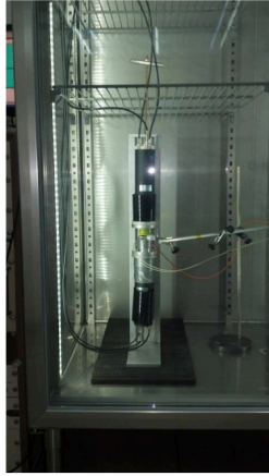
Figure 4 PALS scheme based on a conventional fast-fast coincidence system and picture of the bio-PALS system (the part corresponding to the sample holder, scintillators and photomultipliers) installed inside the refrigerator.
