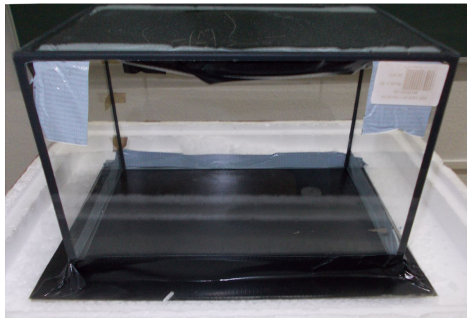
Figure 1.4: Usual design of a home-made cloud chamber. The chamber in the image is the one that was built as part of this thesis.
