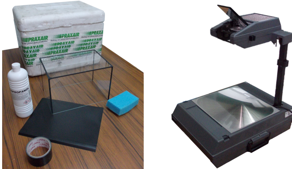
Figure 4.1: Elements used for building the home-made cloud chamber. The dry ice is inside the box at the background of the left image. In subsequent tests, other sponges and plates were also used.
