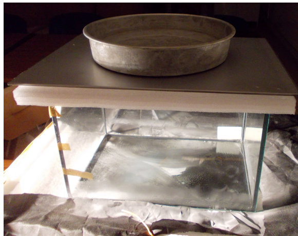
Figure 4.3: Configuration with a heat source on top. The white foam was holed to allow direct heat transfer between the source and the reservoir.
