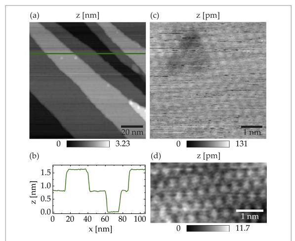
**Figure 5.** (a) Constant current STM topography data resolving several steps with heights of ≈0.8 nm, see (b). (c), (d) The atomic resolution images show a regular hexagonal lattice. In (c) a triangular shaped defect can be identified. The image in (d) is low-pass filtered. The distortion of the hexagonal lattice is due to lateral drift and creep. Imaging parameters: (a) I = 100 pA, U = -800 mV; (c) I = 50 pA, U = 300 mV; (d) I = 100 pA, U = -600 mV;  $T \approx 295$  K.
