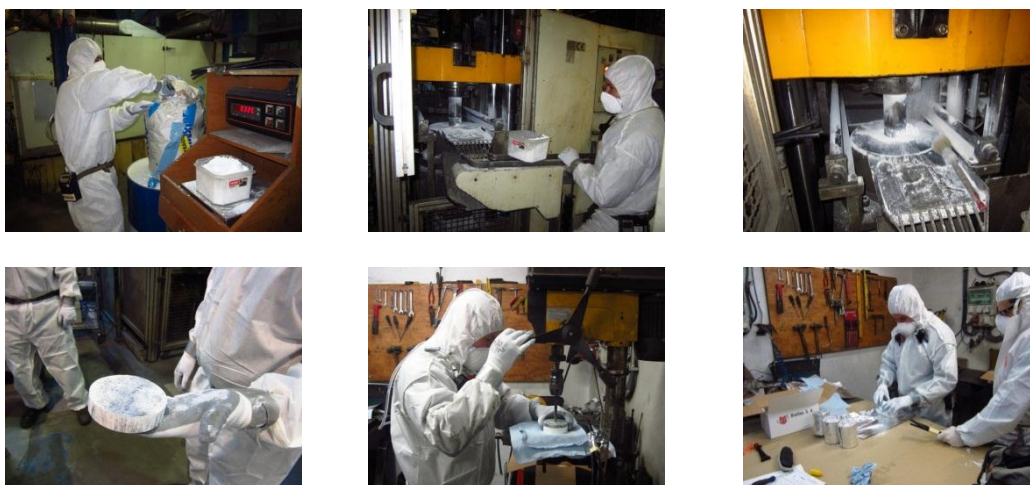
Figure 2. From left to right and top to bottom: 1) Weighing \text{TiO}_2 powder (T1); 2,3) Cold pressing of \text{TiO}_2 powder at vertical axis press (T2); 4) Resulting \text{TiO}_2 tablet at the end of machine cycle; 5) Drilling tablets (T3); 6) Packaging in lots of 5 tablets (T4).
