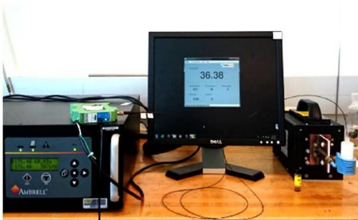
Figure 4. 11 Magnetic hyperthermia system employed. Generator on the left and radio frequency amplifier on the right.
