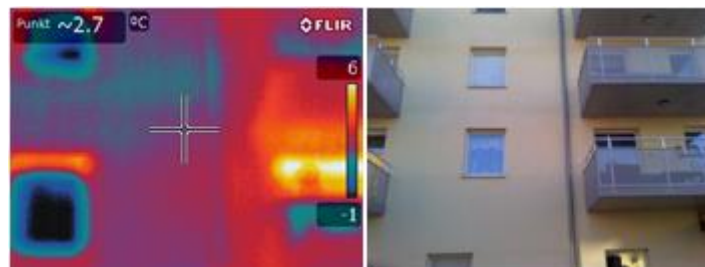
Figure 25: The thermal bridge in a window
