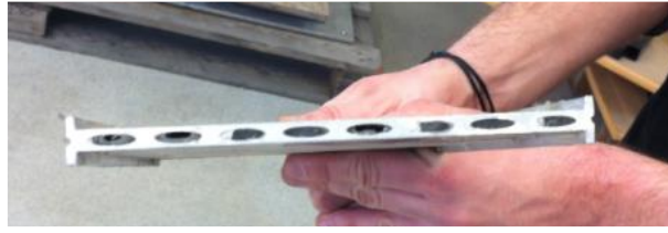
Figure 3.7. Cross section of the Solarus PVT collector's absorber
