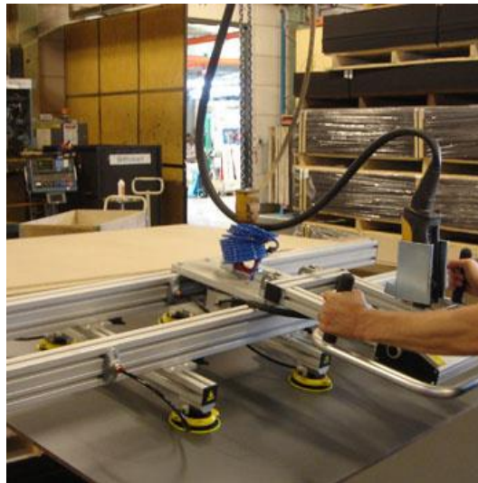
Figure 6.29. Vacuum machine similar as the one used in Absolicon Solar Collector AB [49]
