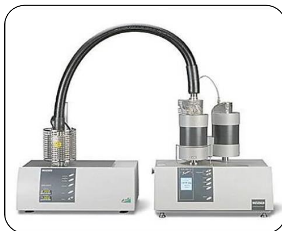
Figure 2.18: The TG-DSC instrument used for measurements.
