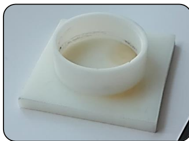
Figure 2.4: PTFE disc for casting of PEO: LiTFSI mixture.
