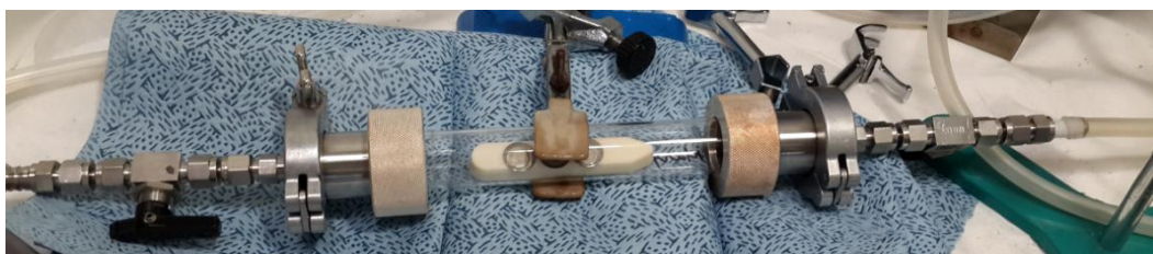
Figure 3.3: Sealed assembly designed for nitridation.
