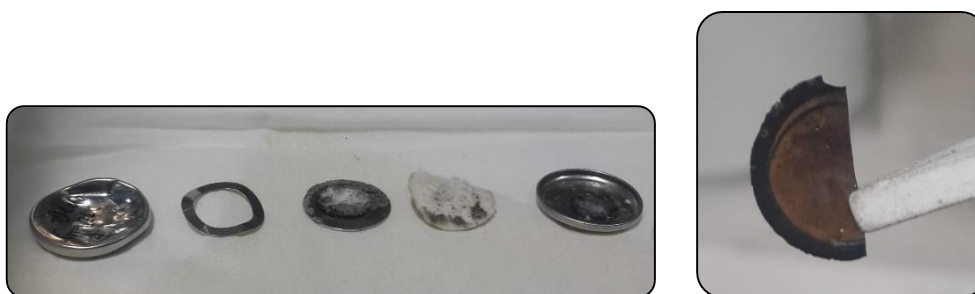
Figure 4.4: A photograph of coin-cell post-mortem and graphite film displaying colour change from black to marron over discharging with Li-anode in presence of 1M LiTFSI (DME:Diox).
