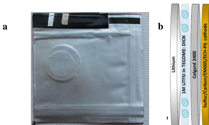
Figure 2.8: a) Photograph of a Li-S coffee bag cell. b) Schematic presentation of the liquid Li-S battery configuration.
