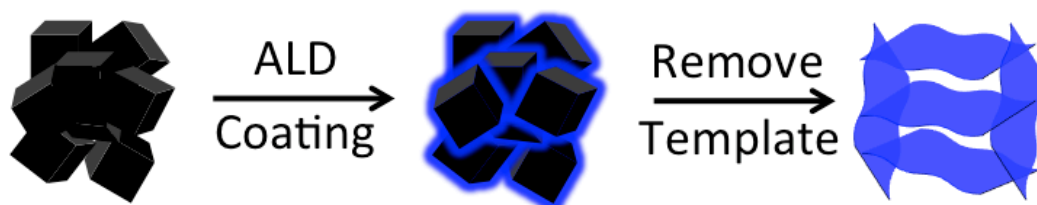
Figure 3.8 Schematic of synthesizing nanosheets by ALD.
