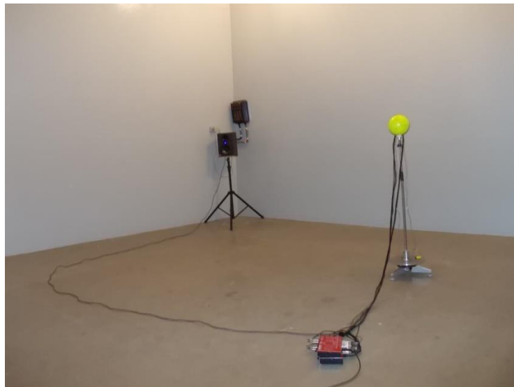
Figure 51. Setup in the reverberant room without absorbing material
