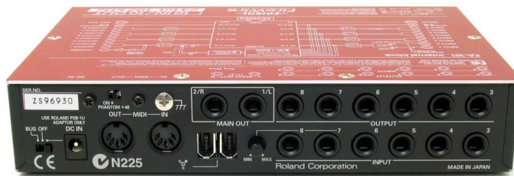
Figure 14. Back of the Edirol FA-101 FireWire Audio Capture [14]
