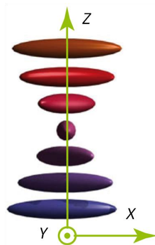
Fig. 1. CLC director configuration. x , y and z are the coordinate axes in the laboratory reference system.
