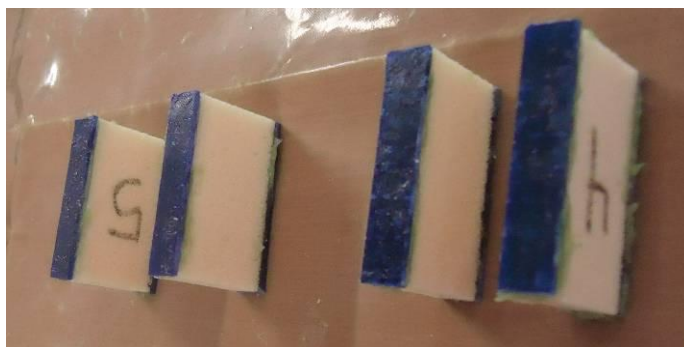
Figure 4.25.- Fabrication of the epoxy sandwich panel.
