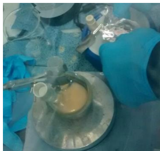
Figure 2.3. A mixture of manganese chloride and lithium carbodiimide inside the glovebox.
