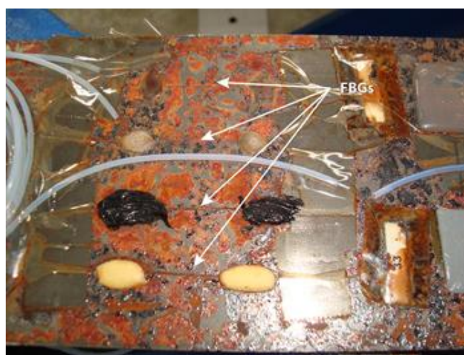
Figure 3. Photograph of four FBGs bonded with different adhesives to the F114 steel specimen after being aged for two months in a climate chamber.
