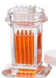
Figure 4.2. Clay films immersion inside staining cuvettes.
