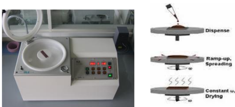
Figure 4.1. (Left) Spin-Coating equipment BLE Spinner Delta 10 and (Right) the thin film elaboration scheme.
