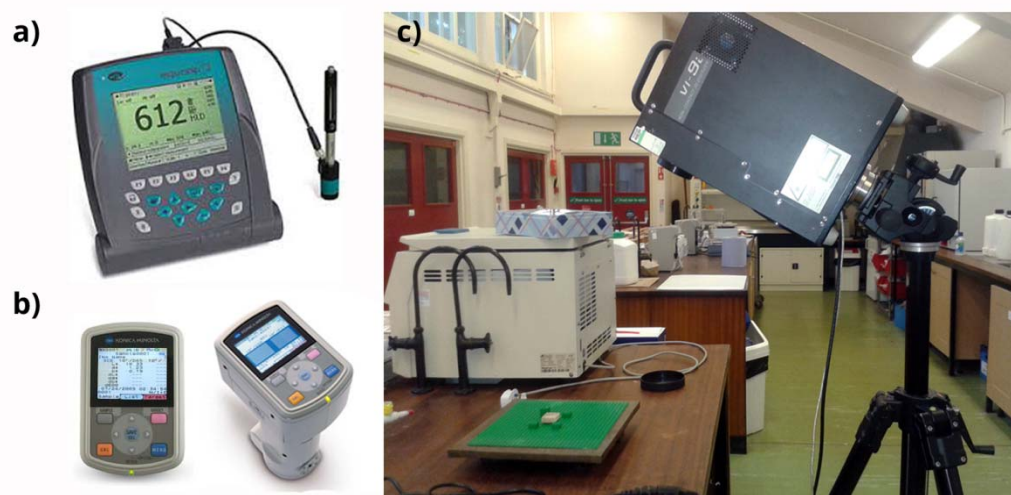
Figure 3.3. Images of portable analytical equipments used to measure physic parameters. a) Rock surface hardness rebound device, Proceq Equotip 3. b) CM-700d Spectrophotometer of Konica Minolta Sensing. c) HD-laser scanner, Konica Minolta (VI-91 3D Digitizer).
