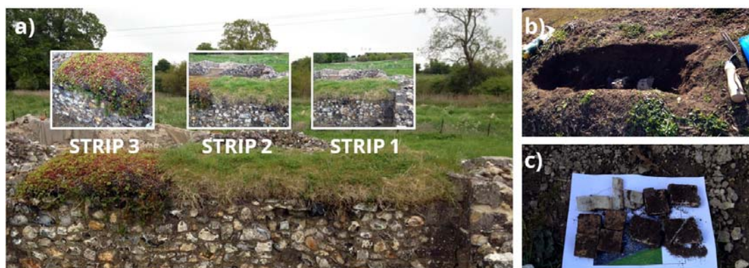
Figure 7.9. a) The wall after one year of soft caps application, where the state of each strip can be observed. b-c) extraction of the samples.
