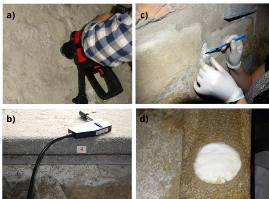
Figure 3.1. Images of the sampling procedure. a-b) Examples of in situ spectroscopic studies, assisted by Raman and DRIFT, taken place previously to the sample collection. c) Collection of an efflorescence sample .d) Extraction of soluble salt content through a cellulose poultice.
