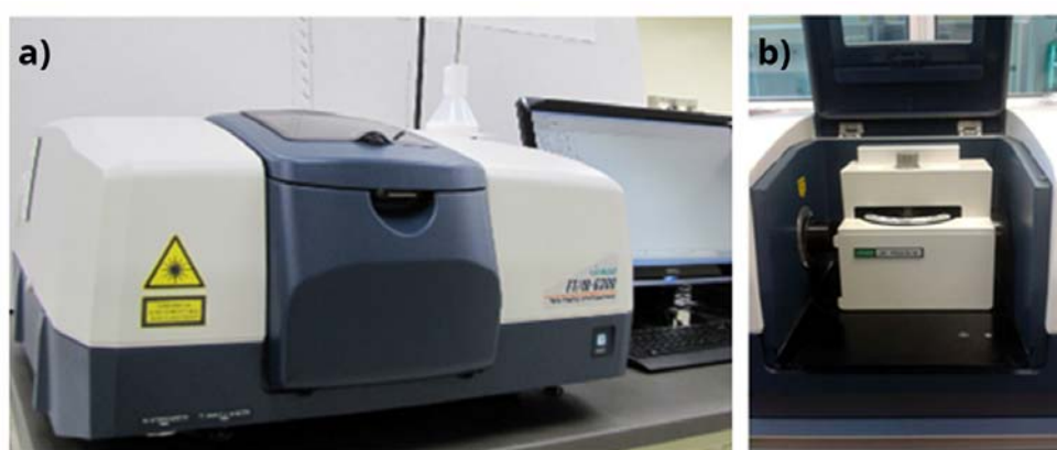
Figure 3.7. Images of DRIFT laboratory equipment. a) FTIR spectrophotometer, 6300 Jasco. b) Difuse reflection module, DR PR0410M Jasco.
