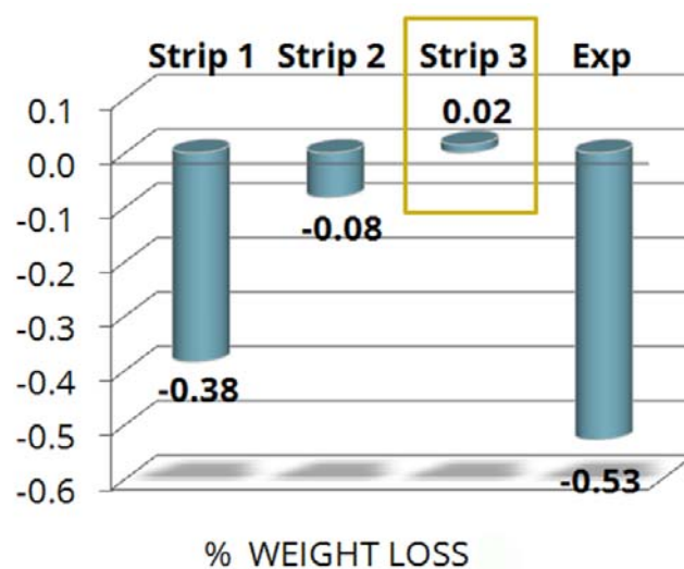
Figure 7.25. Percentage comparison of weight loss average produced under each kind of experiment, in which the values of the open air samples (Exp) correspond to 9 months of exposition and the rest of them to 24 months.
