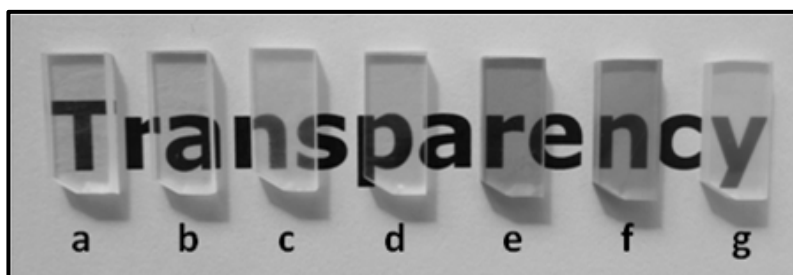
Figure 7.3. Visual appearance of the neat DGEBA-MCDEA cured system (a) and 5 (b), 15 (d) and 25 (f) wt % PS- b -PMMA/(DGEBA-MCDEA) cured systems prepared by the non-solvent method and 5 (c), 15 (e) and 25 (g) wt % PS- b -PMMA/(DGEBA-MCDEA) cured systems prepared by the solvent method.
