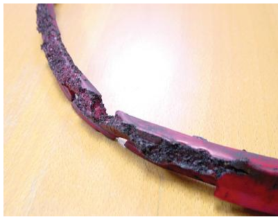
Figure 11: Dieseling damage on a seal (Source: [11]).
