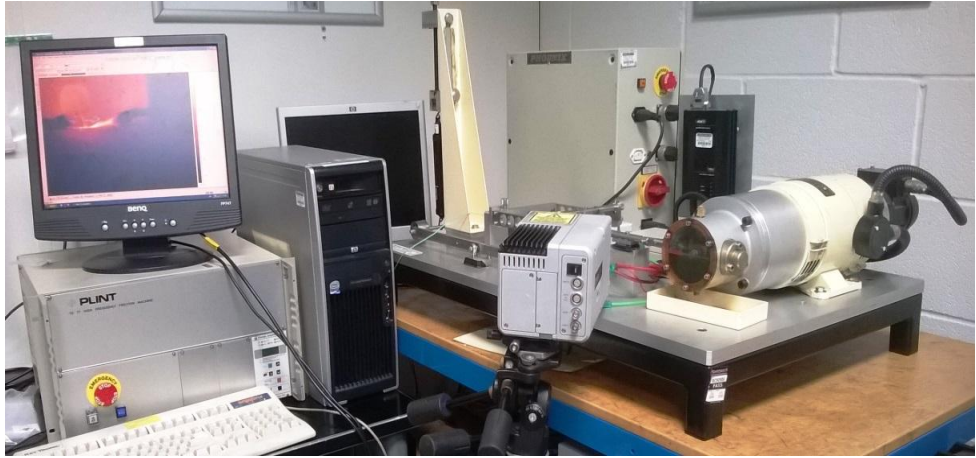
Figure 80: TE77 high frequency sliding test rig (Plint tribology).
