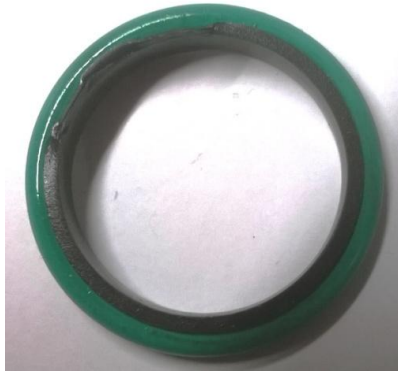
Figure 12: Seal damage due to an incorrect mounting (Source: IK4-Tekniker).
