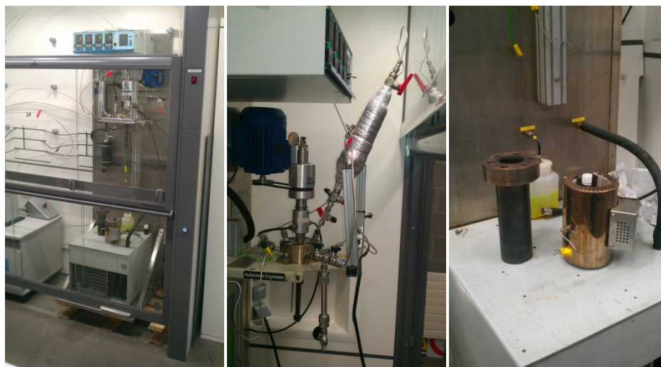
Figure 4.1. Bench scale plant (left), detail of the top of the reactor (center) and the 300 mL reactor and heating jacket (right).
