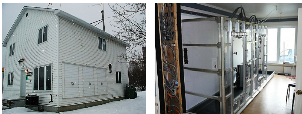
Figura I.14 – FEWF, Field Exposure Wall Facility, del NRC-IRC de Canada
