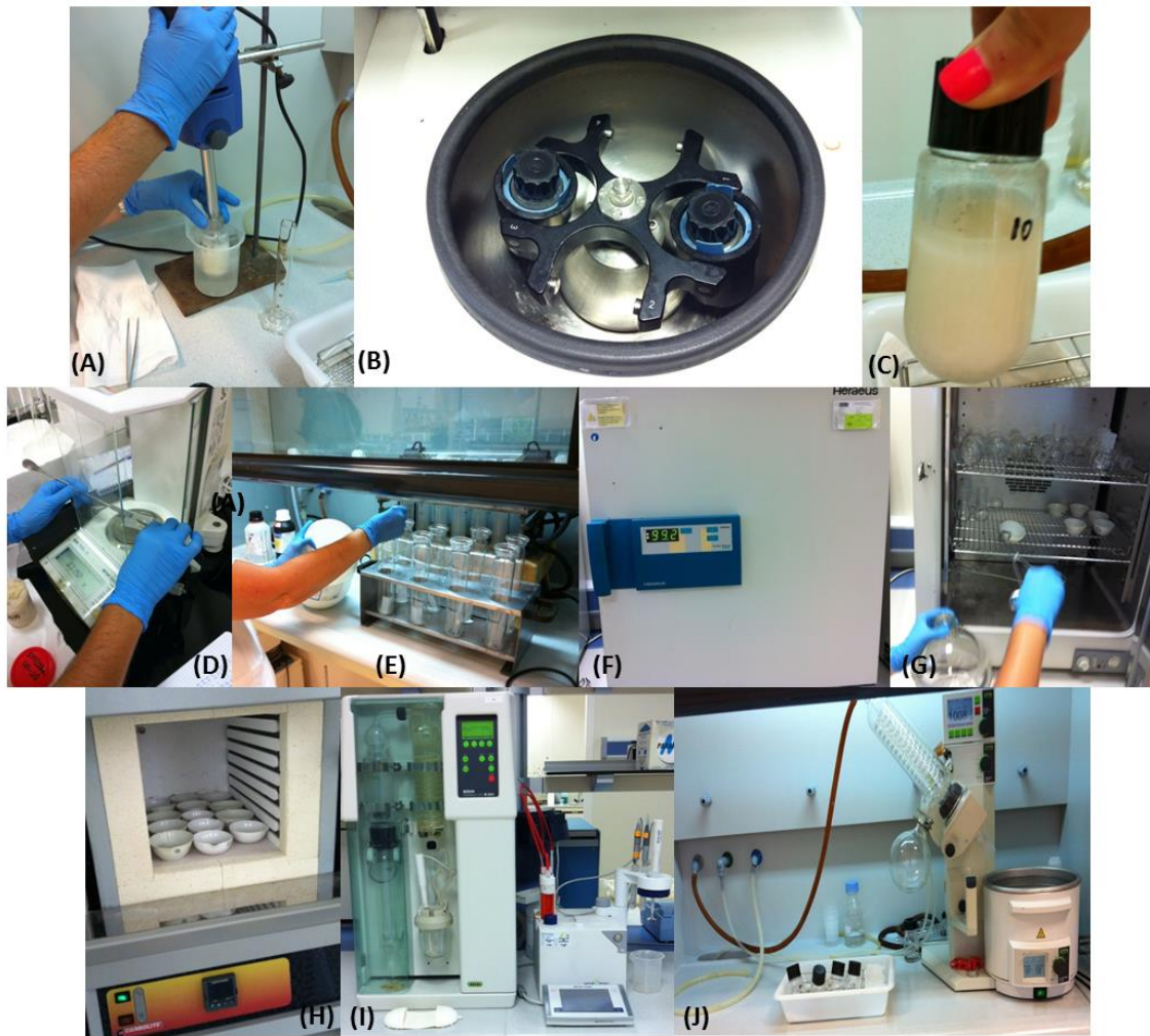
Fig. M.5. Cod and salmon analytical working pictures at the laboratory: (A) whipping the muscle samples for lipid extraction; (B) spinning the whipped sample; (C) sample ready to analyze; (D) weighing sample for protein extraction; (E) digester during the protein extraction method; (F) and (G) Heraeus furnace; (H) humidity determination oven; (I) Kjeldahl distiller with an automatic valuator for nitrogen and protein evaluation; (J) lipid extraction method.
