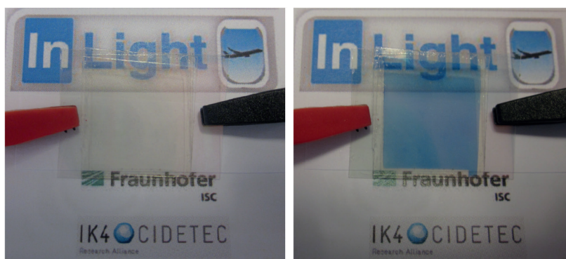
Figure 3.11. Colorless-to-blue switching of an ECD based on [Bn-PO 3 H 2 -Vio]-modified TiO 2 electrodes on ITO/PET cured at 120 °C.
