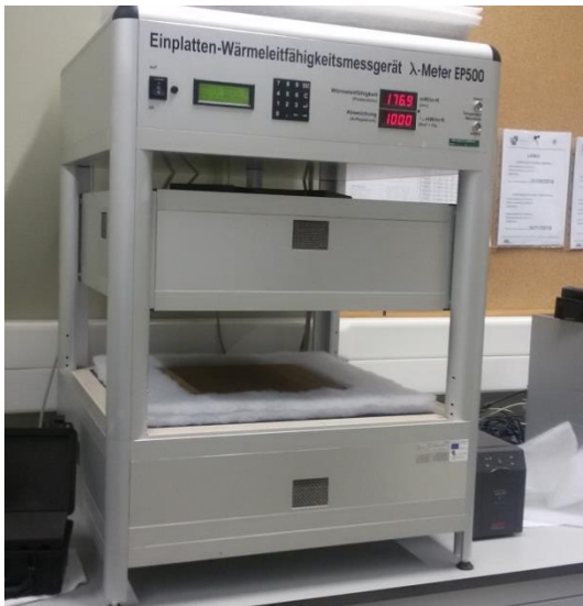
Figure 3.4. λ-Meter EP-500, thermal conductivity measure equipment
