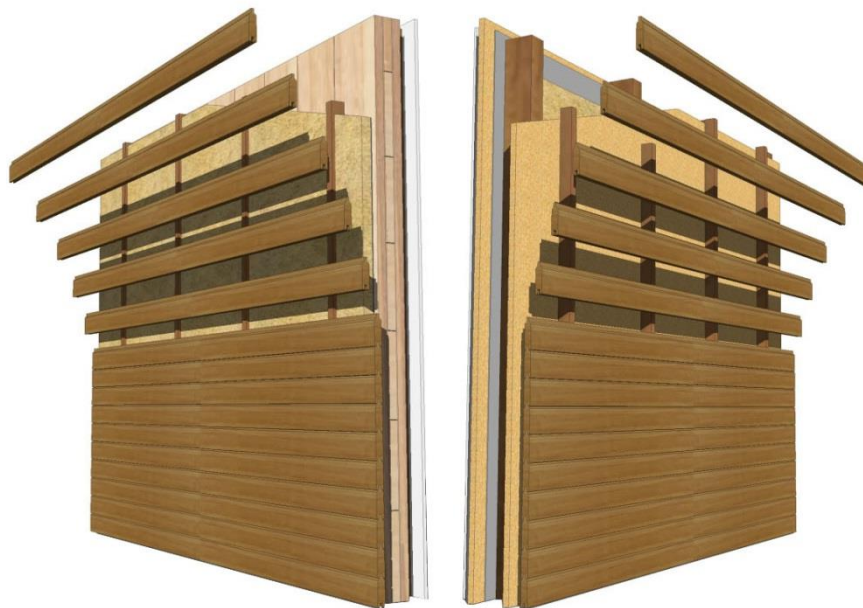
Figure 4.1. CLT (left) and timber framed (right) façades
