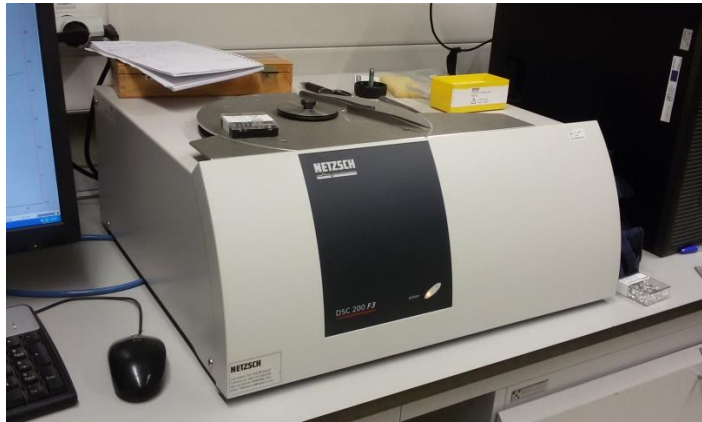
Figure 3.10. NETZSCH DSC 200 F3 Maia equipment
