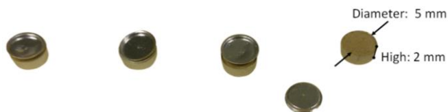
Figure 3.11. Chemical treated Radiata-pine samples
