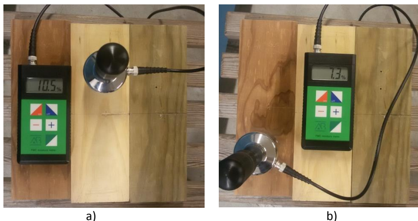
Figure 3.13. Relative humidity measures for natural (a) and heat-treated wood (b)
