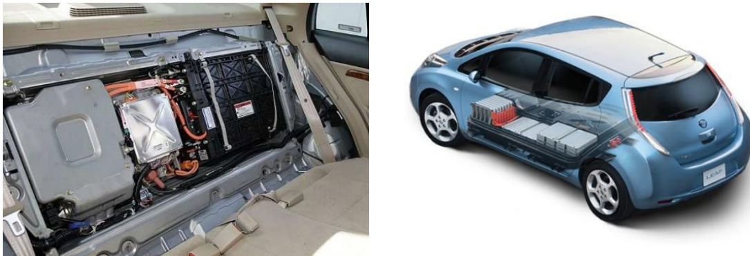
Figure 4.11 (a) Honda Civic BP located in the rear of the back seat [57] and (b) Nissan Leaf BP placed below the seats[56].
