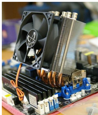
Figure 4.6 Heat pipe system used for cooling a CPU combined with heat sinks and air FC.
