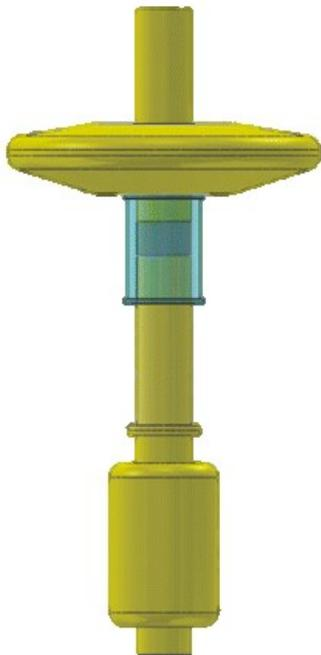
$$\begin{aligned} (m_1 + A_{\infty,11})\ddot{x}_1(t) + A_{\infty,12}\ddot{x}_2 \\ = F_{exc,1}(t) - R_{11} - R_{12} - \rho_w g S_1 x_1(t) \\ + \Delta p S_2 \end{aligned}$$
