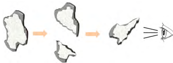
Figure 3.9. Schematic procedure for the salt-slag interface analysis.
