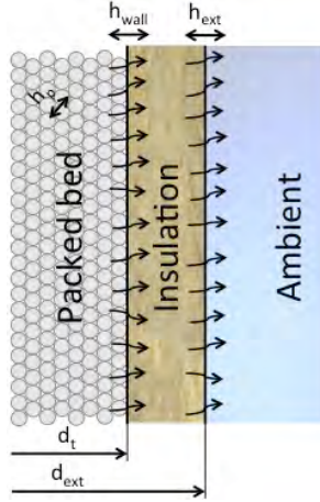
Figure 4.3. Schematic description of the thermal losses.
