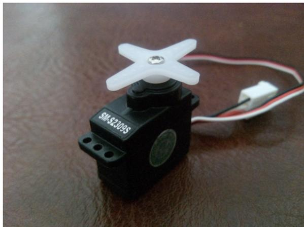
**Figura 3.8:** Servomotor SpringRC SM-S2309S
