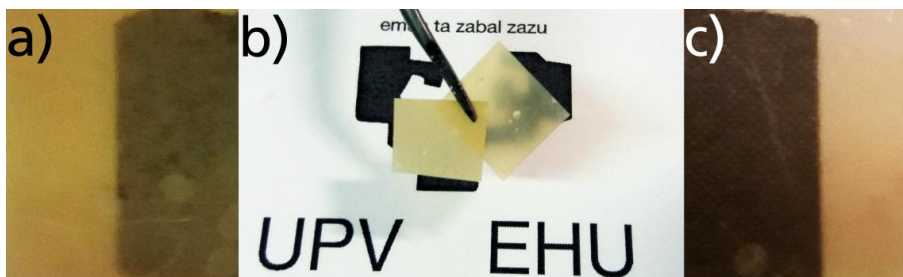
Figure IV-5 Visual aspects of the elaborated CNF-ATS films a) before pressing, b) before and after pressing and c) after pressing.
