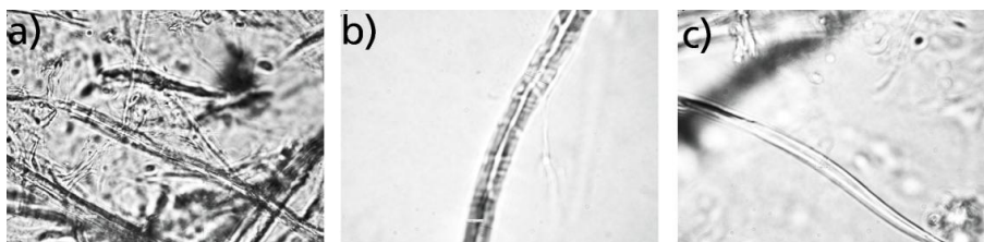
Figure I-20. Different fibrillation grades as view with O.M. with 200x.
