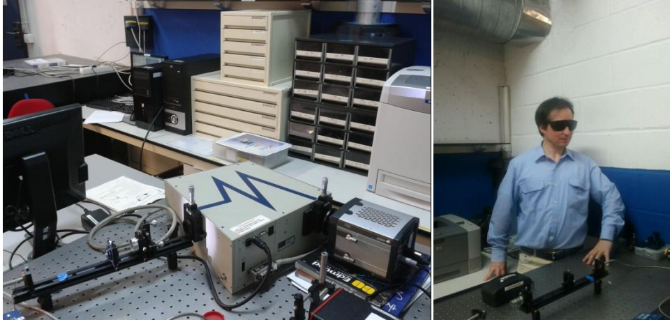
Figure 2.9. Laboratory layout including radiative source, monochromator and sCMOS detector
