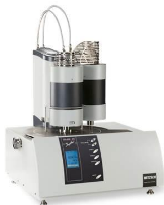
Figure A.5 a) NETZSCH Simultaneous Thermal Analyzer (STA) 449 F3 Jupiter® and b) Scheme of a thermobalance 12 .
