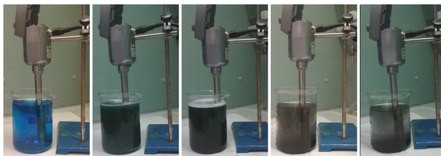
Figure 4.6: Evolution of reduction-oxidation reaction over time: a) before adding graphite nanoplates, b) 0 minutes, c) 10 minutes, d) 25 minutes and e) 35 minutes.
