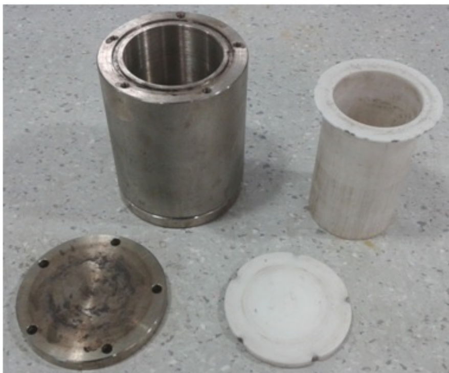
Figure 4.14: Image of the custom-made autoclave used in the hydrothermal synthesis.
