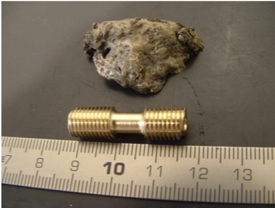
Figure 4.19: Sample image of a testing tube made out of GNP/ZrO 2 and bronze MMC.
