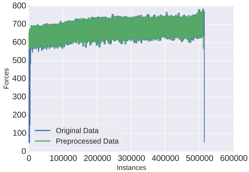
Fig. 2: Original data versus Filtered Data for Inconel 718, LGA, HPC, T2, pass 1.
