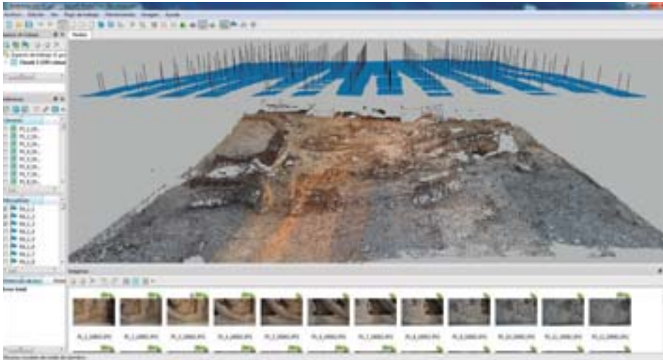
Figure 5. Screenshot of the software PhotoScan. As in Figure 3, the perspective view shows together the point cloud representing the surface of the site and the location of the cameras (blue quadrilaterals).
