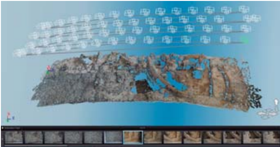
Figure 3. Screenshot of the software 123D Catch, in which a three-dimensional view of the terrain model is presented in form of point cloud. The location of the cameras is also shown. The model corresponds to four strips (59 pictures).
