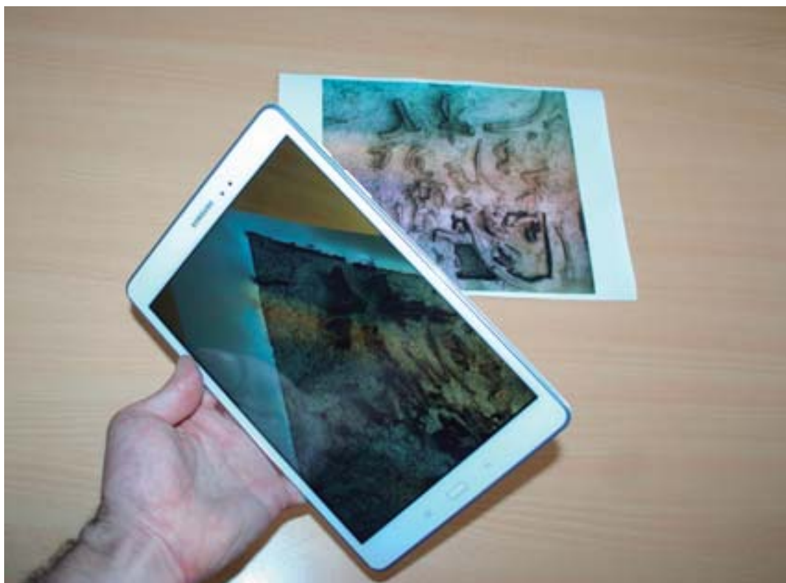
Figure 10. Interactive view of the 3D model in a tablet. The piece of paper with the orthoimage of the site acts as the marker on which the 3D model is placed.
