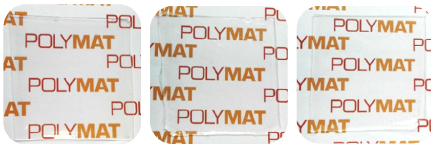
Figure III-10. Pictures of polymer films containing (from left to right) 20, 30 or 40 wbm% methacrylate fructose.
