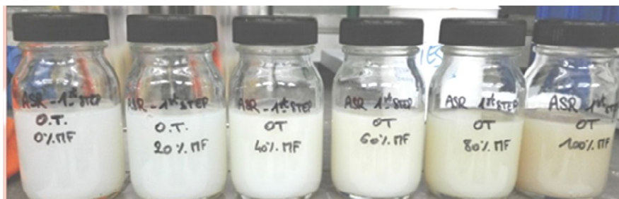
Figure V-9. Picture of the different ASR solutions after neutralization (from A-MF0 on the left to A-MF100 on the right)
