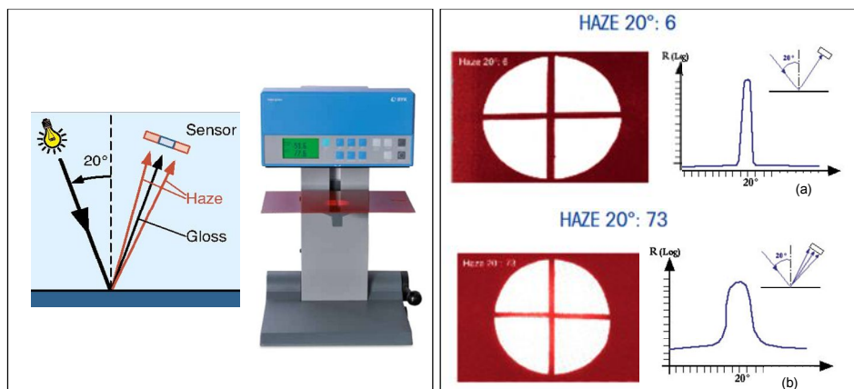
Figure IV-2. Representation of gloss and haze film measurement
