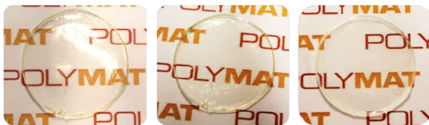
Figure III-9. Pictures of polymer films containing (from left to right) 20, 30 or 40 wbm% methacrylate galactose content.
