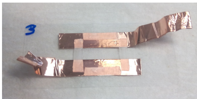
Figure 2.13. Electroporation chamber used in this study. The chamber is made of a rectangular glass coverslip where two copper stripes have been stuck 0.5 cm apart. Heated parafilm was used to create a cavity for deposition of the sample. The cavity was then covered with a smaller square coverslip.
