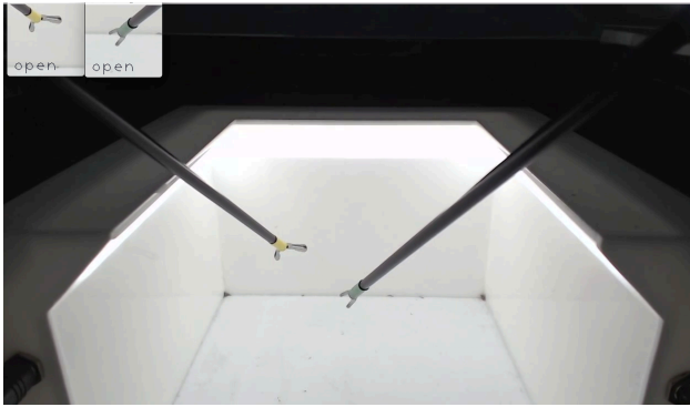
Figure 8. Screenshot of an evaluation with two laparoscopic instruments, showing the complete image and regions of interest labeled with the current predicted state of clamps' aperture.
