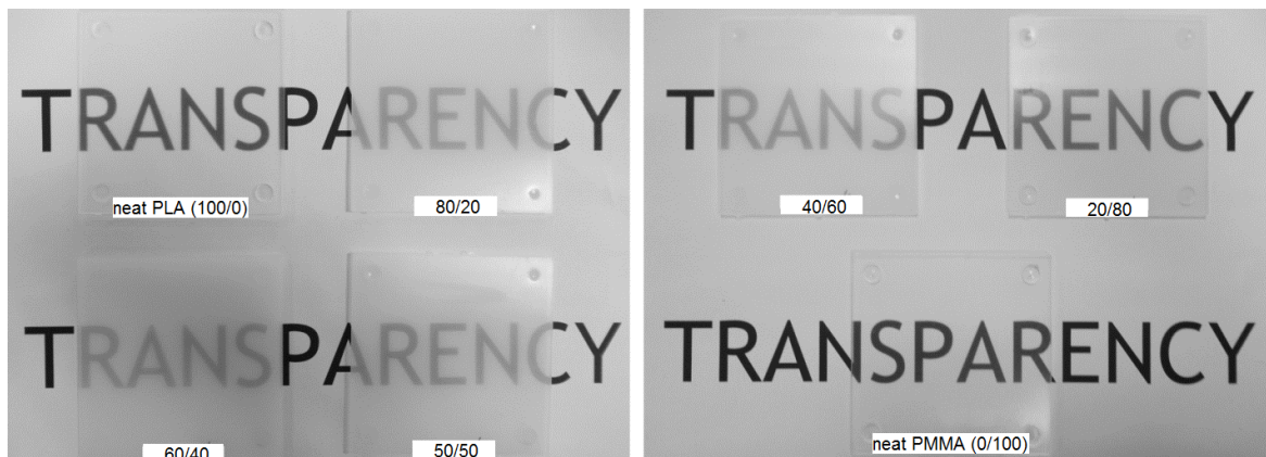
Fig. 3-4. Injection moulded platelets for all systems.
