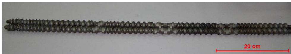
Fig. 3-2. Screw configuration used for melt compounding.
