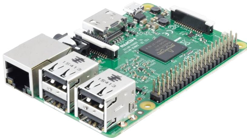
*Figura 7. Raspberry Pi 3 (Modelo B)*
